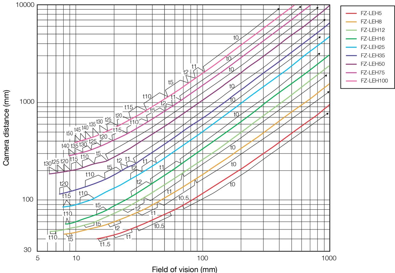
The 5-mm Extension Tubes (3Z4S-LE ML-EXR) cannot be used with FZ-LEH25 Lenses.
