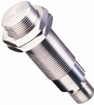
The GS1001-1002 series gear tooth sensors are Hall Effect devices designed for use in applications where ferrous edge detection or near zero speed sensing (without power up recognition) is needed. Current sinking output requires the use of a pull up resistor. Circuit protected with adjustable stainless steel housing
