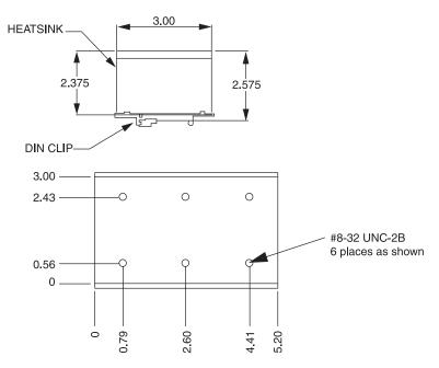
**DIMENSIONS:** inches **TOLERANCES:** ±0.02 inches **MATERIAL:** AISI 6063-T5 Aluminum
