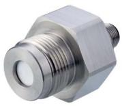
The semi-flush mount pressure transmitter, IPSS, has a piezo-resistive silicon or ceramic pressure sensor. The sensor is semi-flush to the housing making this product ideal for viscous or paste like media. The sensor and housing are made from stainless steel with a choice of internal '0' ring seals to ensure the product is suitable for a wide range of applications.
