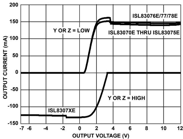
FIGURE 9. DRIVER OUTPUT CURRENT vs SHORT CIRCUIT VOLTAGE
