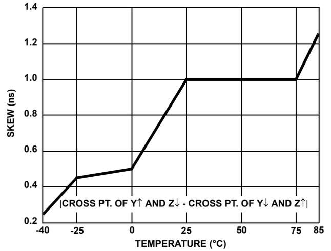
FIGURE 14. DRIVER DIFFERENTIAL SKEW vs TEMPERATURE (ISL83073E, ISL83075E)
