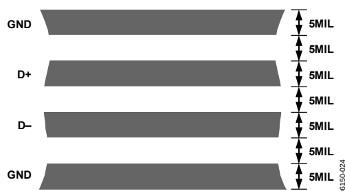
Figure 24. Typical Arrangement of Signal Tracks
