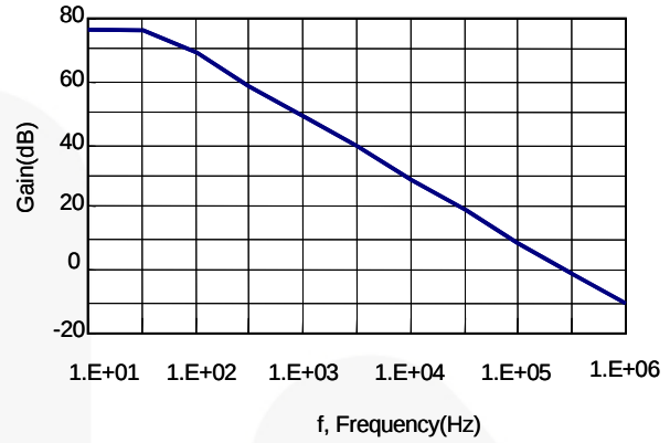
Figure 3. Open-Loop Voltage Gain
