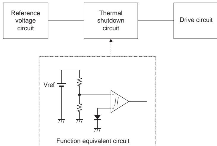
Note: The above is an example of thermal shutdown circuits although there are some differences from the actual internal circuit.
