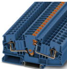
Test disconnect terminal block, Connection method: Spring-cage connection, Cross section: 0.2 mm 2 - 10 mm 2 , AWG: 24 - 10, Width: 8.2 mm, Color: blue
