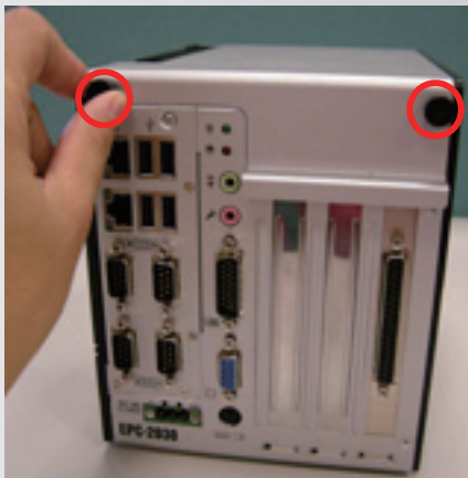
Thumbscrew Design for Easy, Tool-free Installation
