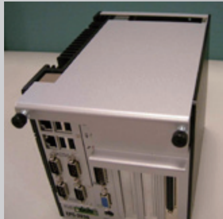
Easily Remove Top Cover by Hand
