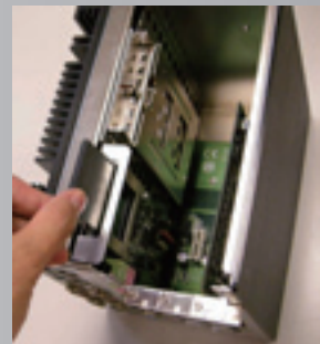
CFast Card Installation
