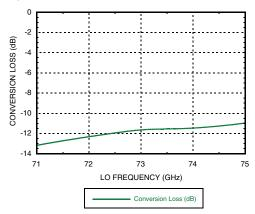
Note 1: Measured Performance Characteristics (T<sub>OP</sub> = 25°C)
