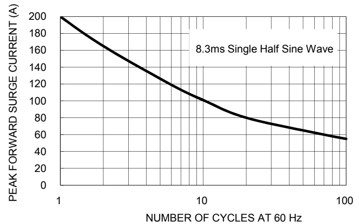
FIG. 2- MAXIMUM FORWARD SURGE CURRENT PER LEG
