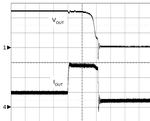
Over Current Protection
