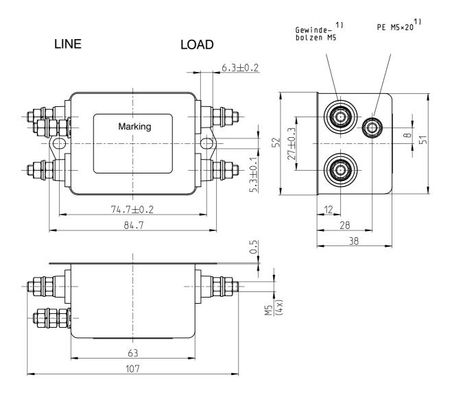
1) Tightening torque 2,6...3,0 Nm!
