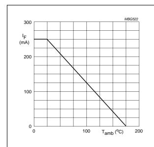
Device mounted on a printed-circuit board without metallization pad.
