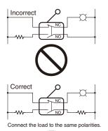
Incorrect Power Connection Example (Connection of Different Power Supplies) There is a risk of AC and DC mixing.
