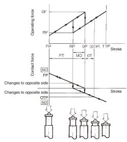
If the Limit Switch is used so that the actuator is constantly pressed, it will fail quickly and reset faults may occur. Inspect the Limit Switch periodically and replace it as required.
