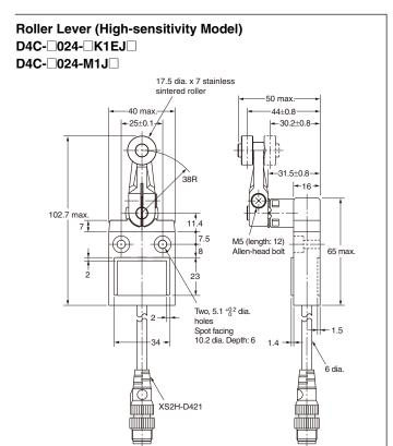
Note: Unless otherwise specified, a tolerance of  $\pm 0.4$  mm applies to all dimensions.
