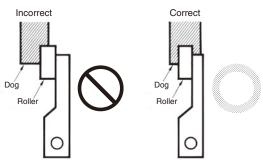
• With a roller actuator, the dog must touch the actuator at a right angle. The actuator or shaft may deform or break if the dog touches the actuator (roller) at an oblique angle.
