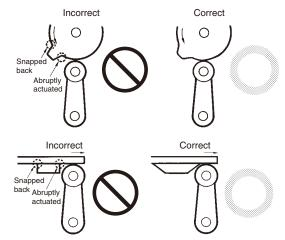
Appropriate force must be imposed on the actuator by the cam or dog in both rotary operation and linear operation.
