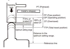
• The Limit Switch may soon malfunction if the OT is excessive. Therefore, adjustments and careful consideration of the position of the Limit Switch and the expected OT of the operating body are necessary when mounting the Limit Switch.
