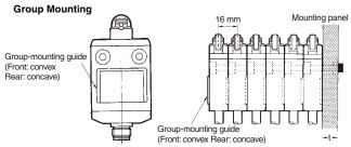
If the mounting panel is warped or has protruding parts, a malfunction may result. Make sure that the mounting panel is not warped and has even surfaces.
