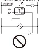
Do not design a circuit where voltage is imposed between contacts, otherwise contact welding may result.
