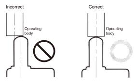
• Be sure to use the Limit Switch according to the characteristics of the actuator.
