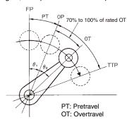
The movement distance of the dog based on the optimum stroke is expressed by the following formula.
