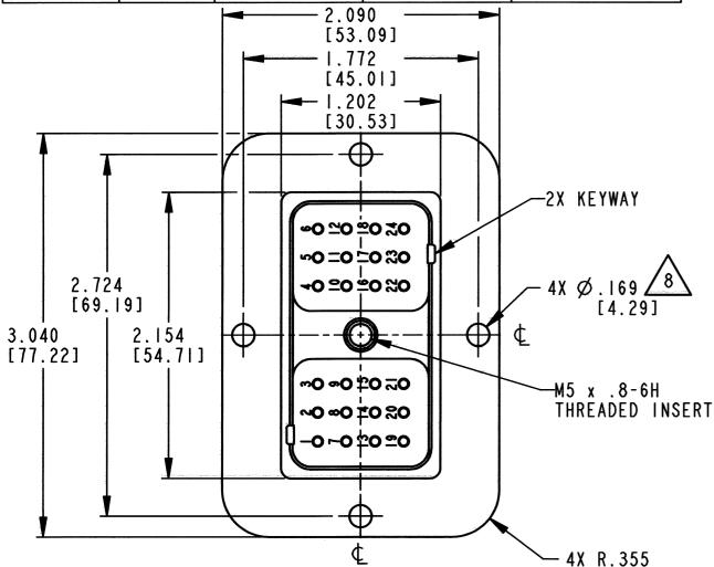
5. THIS PART MATES WITH DRC16-24SA\*-\*\*\*\* PLUG. (\* = WIRE SEAL ID; \*\*\*\*= ALL MODIFICATIONS)
