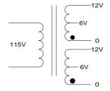
\* Secondary windings are designed to be connected in series or parallel. Windings are not intended to be used independently.
