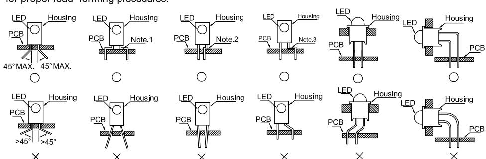
" " Correct mounting method " " Incorrect mounting method
