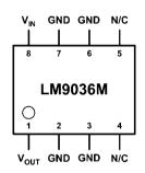
Top View LM9036M-3.3, LM9036MX-3.3, LM9036M-5.0, LM9036MX-5.0 See NS Package Number M08A
