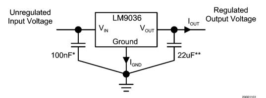
\* Required if regulator is located more than 2 from power supply filter capacitor.
