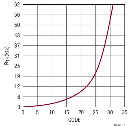
Figure 1. Programmable  $R_{TH}$
