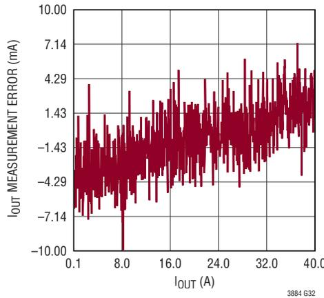
**Input Current Error vs Input Current**
