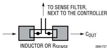
Figure 27. Sense Lines Placement with Inductor DCR
