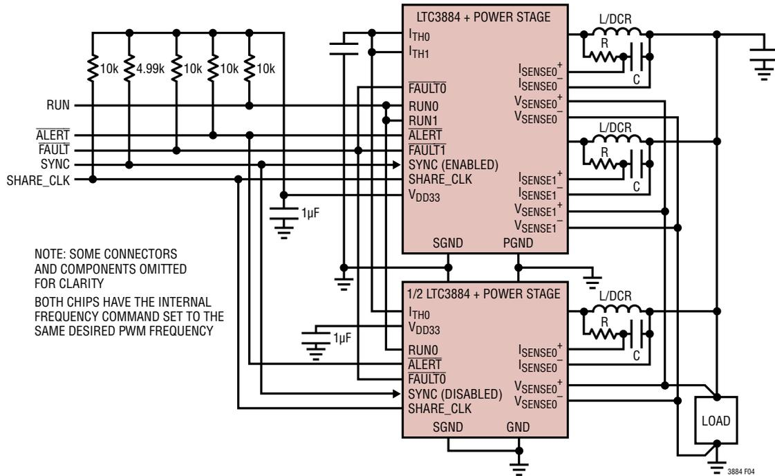
Figure 4. Load Sharing Connections for 3-Phase Operation
