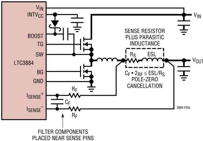
FILTER COMPONENTS PLACED NEAR SENSE PINS
