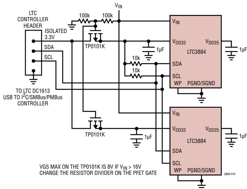
Figure 41. Controller Connection
