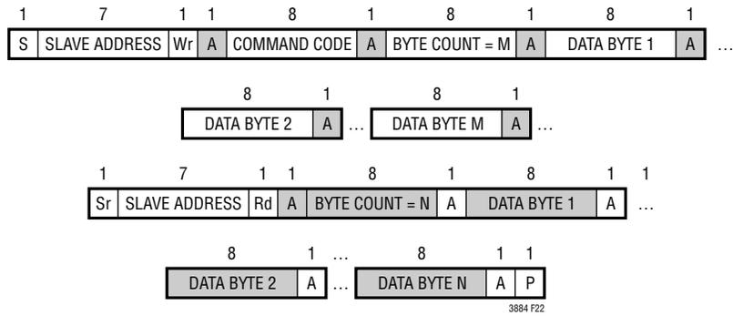
Figure 22. Block Write – Block Read Process Call
