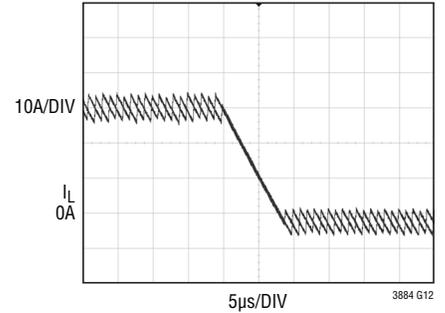
**Dynamic Current Sharing During a Load Transient in a 4-Phase System**
