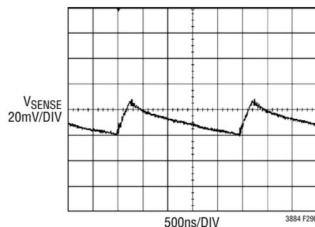
Figure 29b. Voltage Measured After the  $R_{\text{SENSE}}$  Filter
