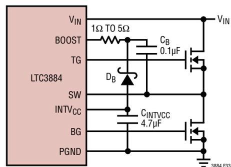
Figure 33. Boost Circuit to Minimize PWM Jitter
