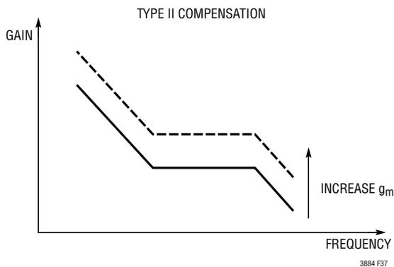
Figure 37. Error Amp  $g_m$  Adjust
