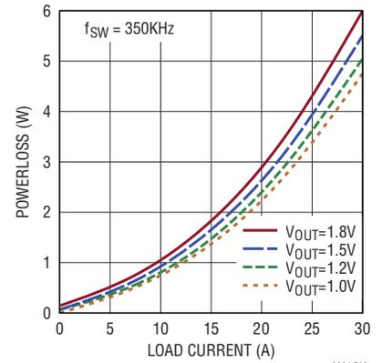
Power Loss vs Output Current
