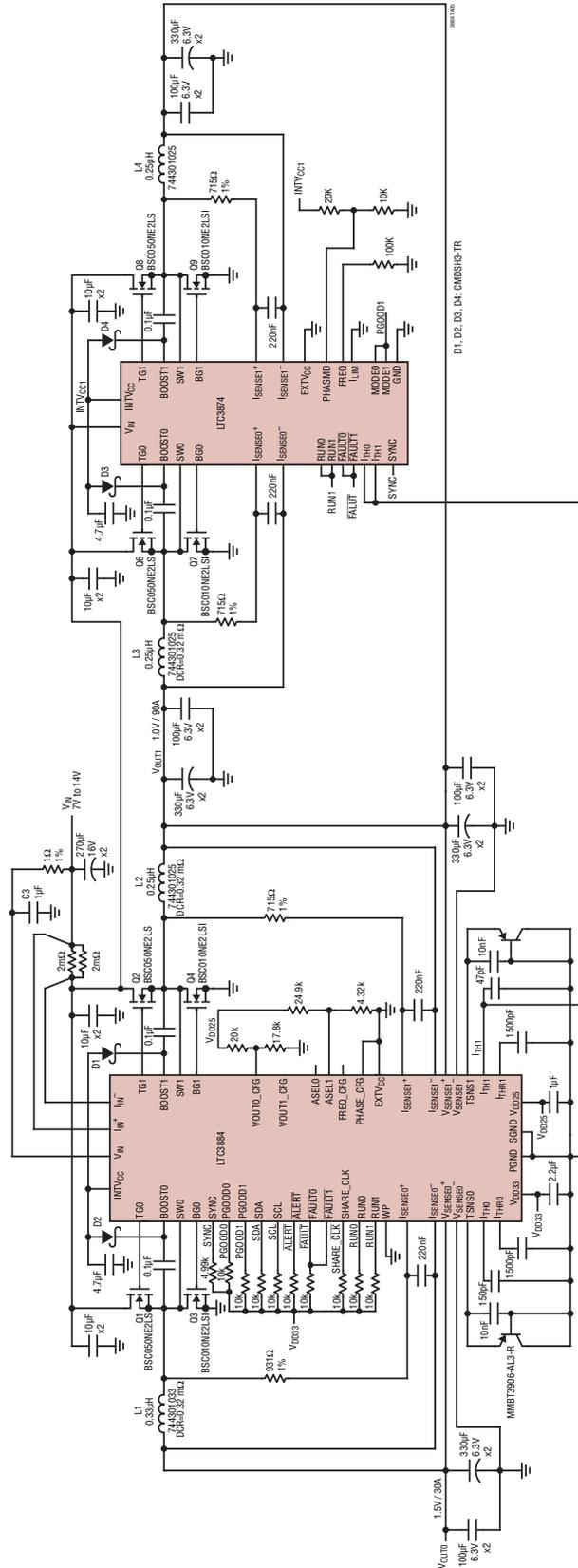
Figure 39. Master/Slave 3 +1 High Efficiency, Dual-Output, 1.5V/30A and 1.0V/90A Buck Converter (LTC3884/LTC3874)
