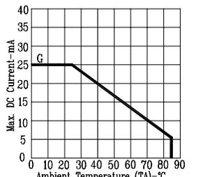
Fig5. MAX. ALLOWABLE DC CURRENT VS. AMBIENT TEMPERATURE.
