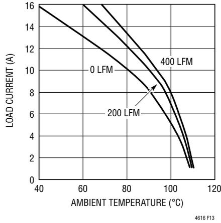
**Figure 13. 3.3V<sub>IN</sub> to 1.2V<sub>OUT</sub> with No Heat Sink**
