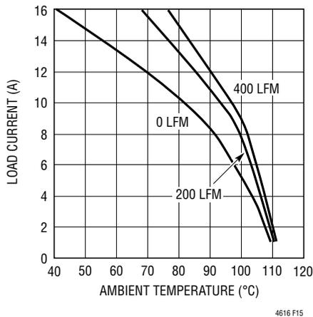
**Figure 15. 3.3V<sub>IN</sub> 1.2V<sub>OUT</sub> with BGA Heat Sink**
