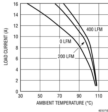
**Figure 16. 3.3V<sub>IN</sub> 2.5V<sub>OUT</sub> with BGA Heat Sink**
