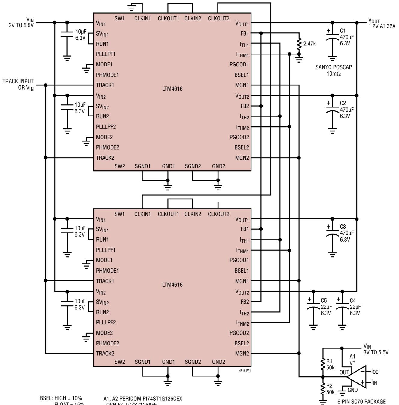
Figure 21. Four Phase in Parallel, 1.2V at 32A
