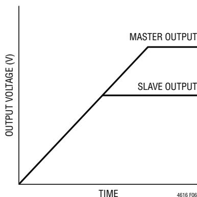
Figure 6. Output Voltage Coincident Tracking
