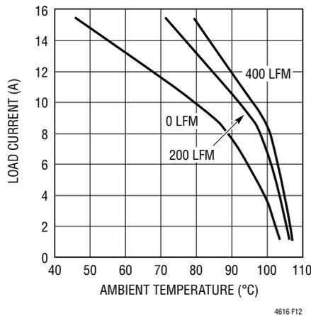
**Figure 12. 5V<sub>IN</sub> to 1.2V<sub>OUT</sub> with BGA Heat Sink**
