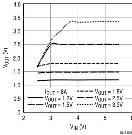
**V<sub>IN</sub> to V<sub>OUT</sub> Step-Down Ratio**
