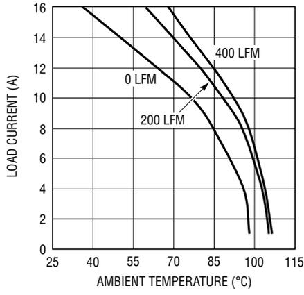
**Figure 9. 5V<sub>IN</sub> to 3.3V<sub>OUT</sub> with No Heat Sink**
