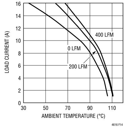
**Figure 14. 3.3V<sub>IN</sub> to 2.5V<sub>OUT</sub> with No Heat Sink**
