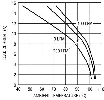
**Figure 10. 5V<sub>IN</sub> to 1.2V<sub>OUT</sub> with No Heat Sink**
