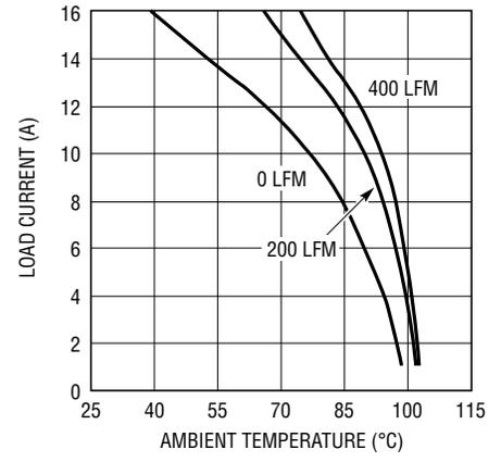
**Figure 11. 5V<sub>IN</sub> to 3.3V<sub>OUT</sub> with BGA Heat Sink**
