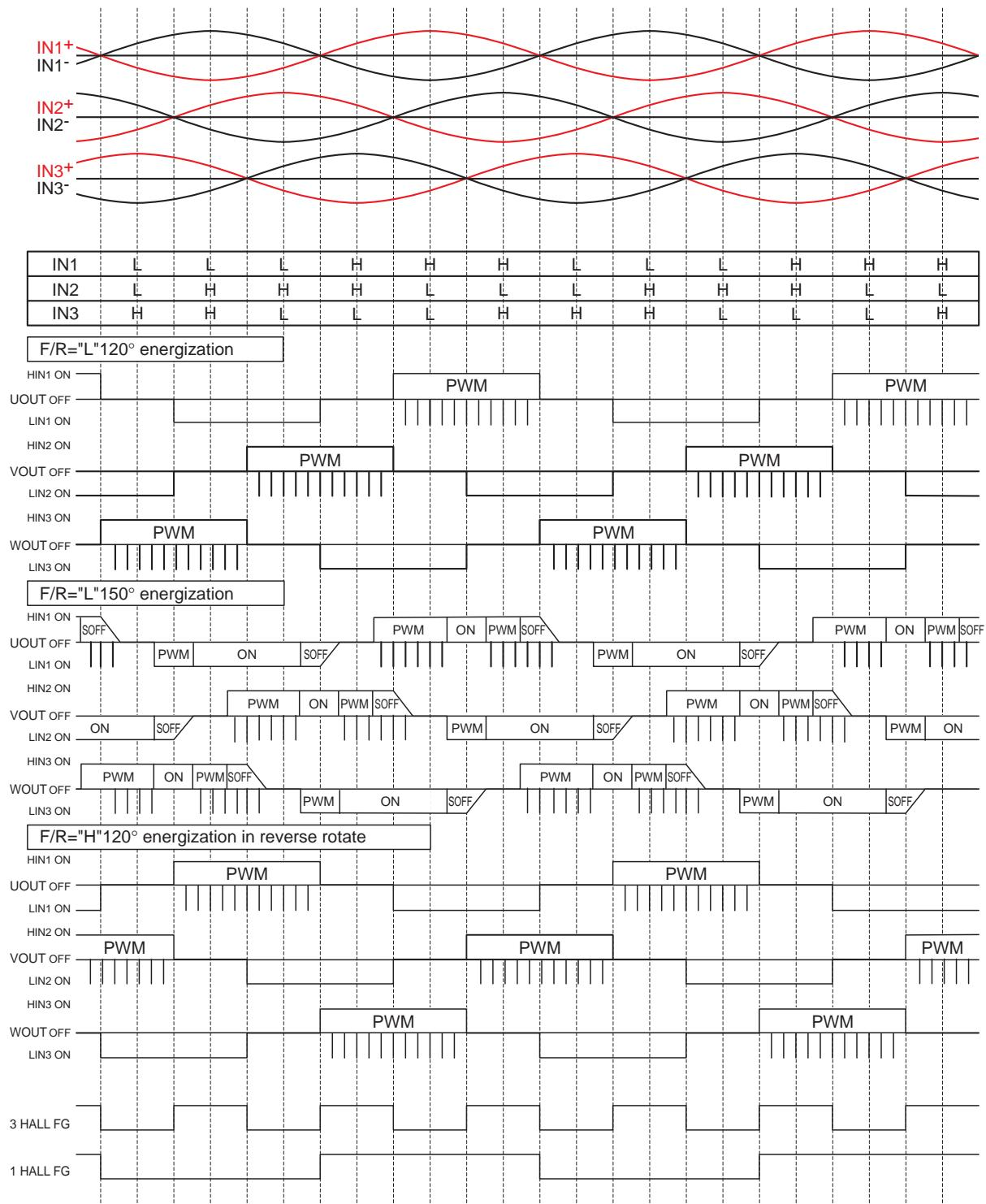
The energization is switched to 120° when 3 Hall FG frequency is 6.1Hz (TYP) or lower
