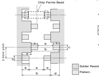
\*As for BLM31PG type, taking land pad thickness and rated current into account.
