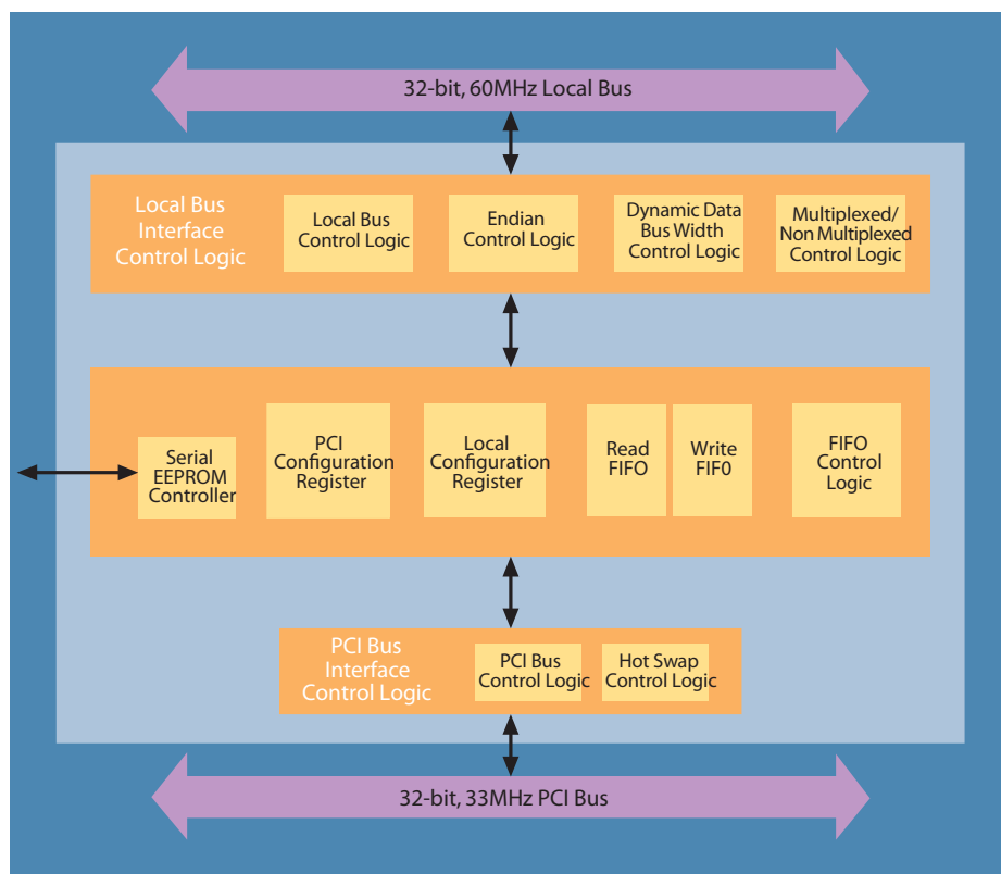
PLX PCI 9030 Block Diagram
