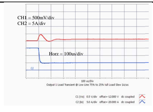
Vo=12V Typical output voltage transient response to load step from 75% to 25% of full load with output current slew rate of 1A/uS. (Cext = 200uF capacitor)
