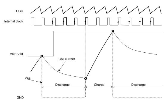
The average current value becomes lower than the set current value because of the peak current detection method. It should be noted that the average current value changes, depending on the motor characteristics.
