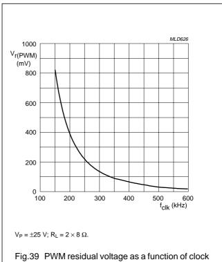
Fig.39 PWM residual voltage as a function of clock frequency.
