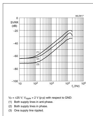
Fig.30 SVRR as a function of input frequency.
