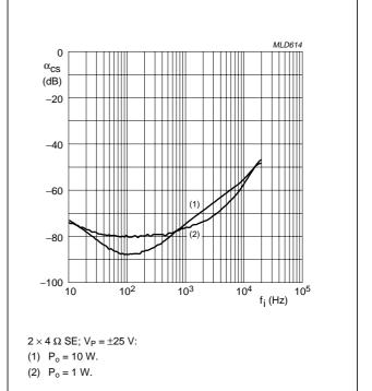
Fig.27 Channel separation as a function of input frequency.
