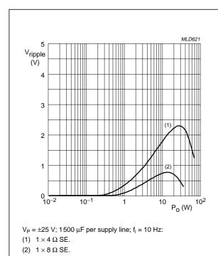
Fig.34 Supply voltage ripple as a function of output power.
