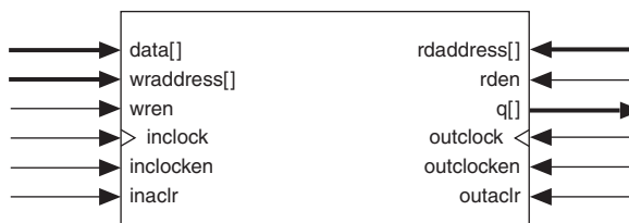
Figure 2–13. Simple Dual-Port and Single-Port Memory Configurations
