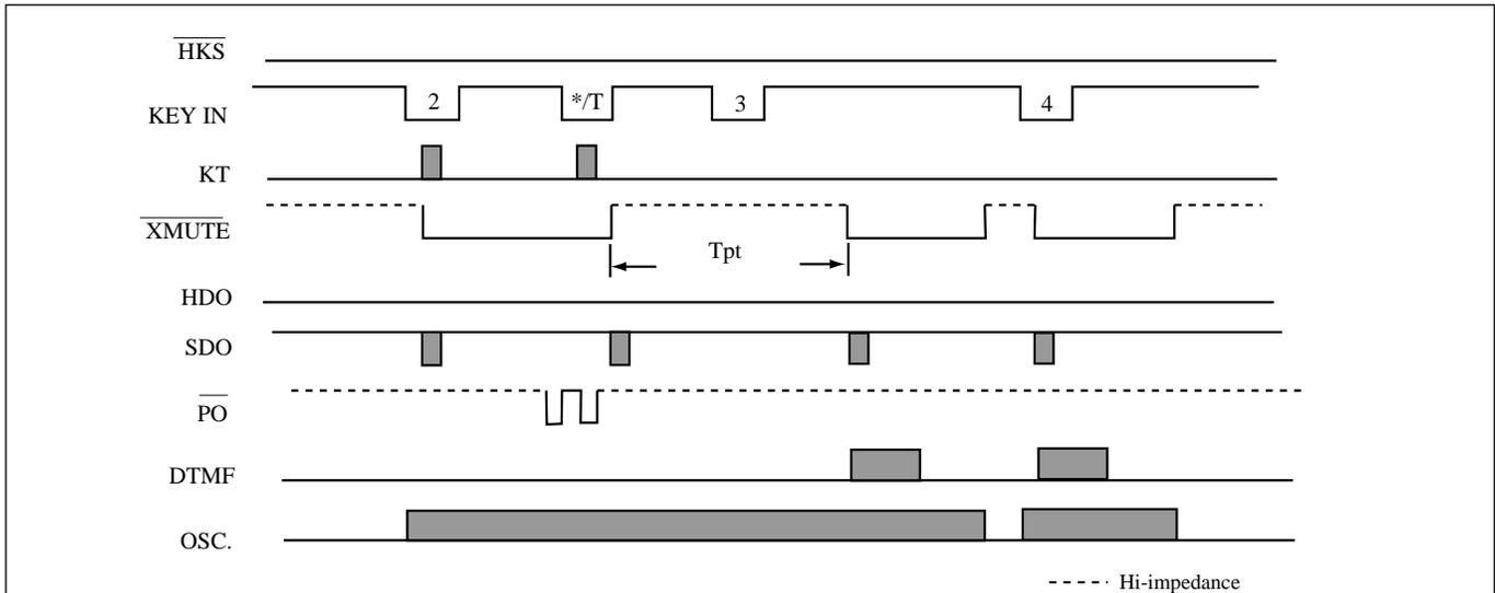
Figure 6. Pulse to Tone (P→T) operating timing
