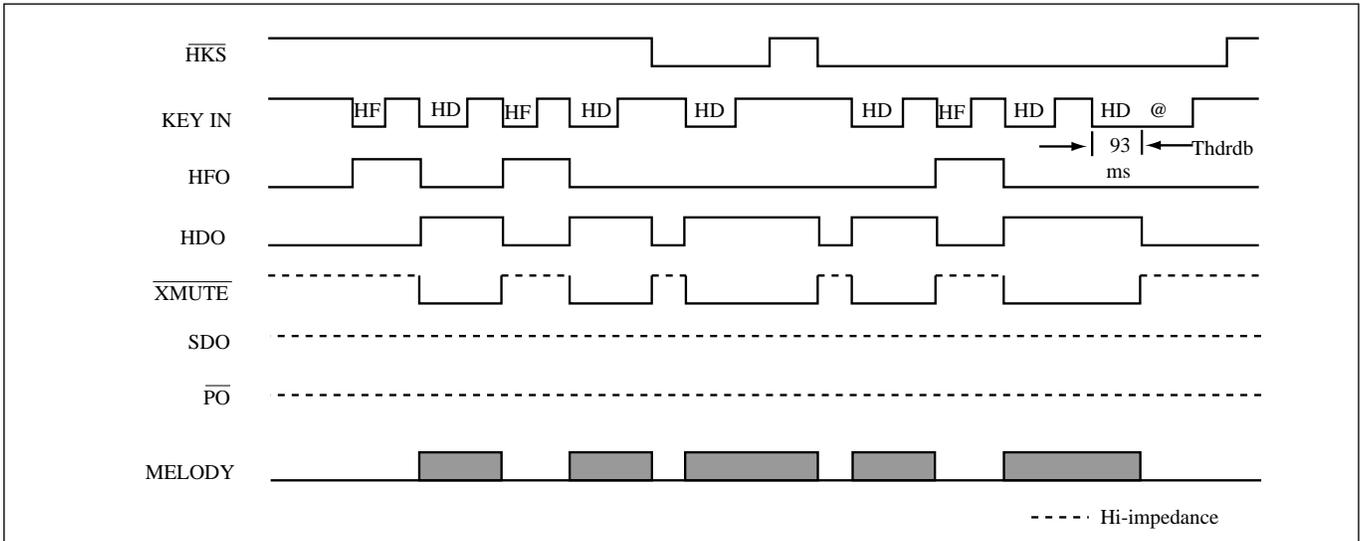
@ : It can be triggered by extension telephone set for hold function release
