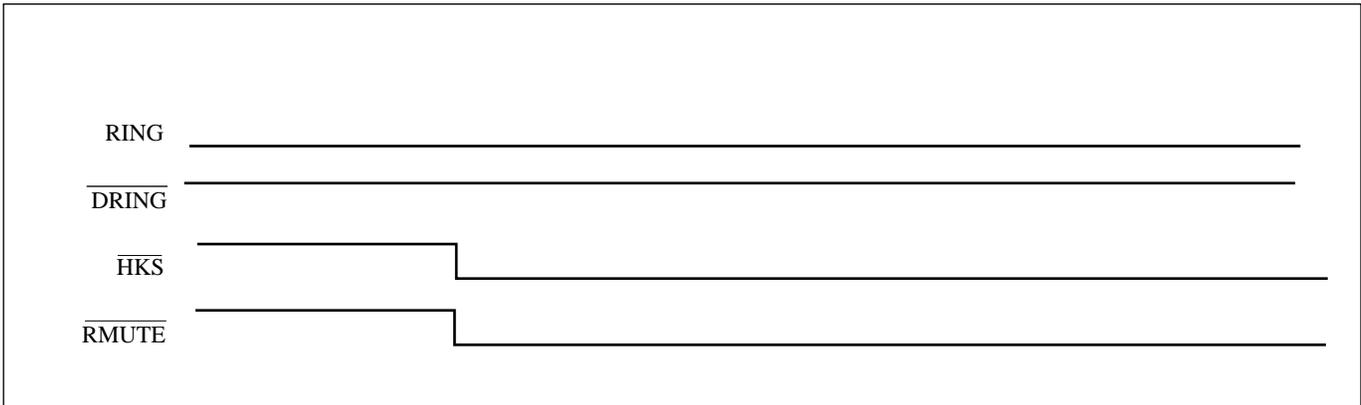
Figure 12. Timing of making an outgoing call
