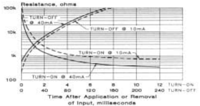
Output Resistance vs. Input Current
