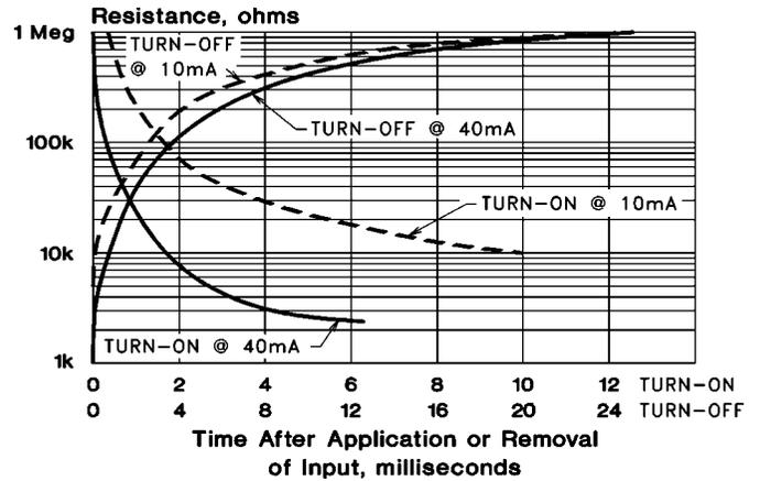
Output Resistance vs. Input Current
