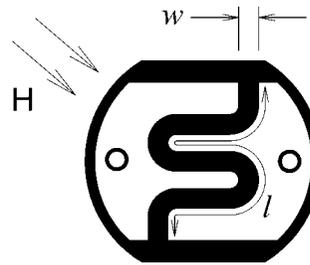
$R_H$  = resistance of cell at light level H
