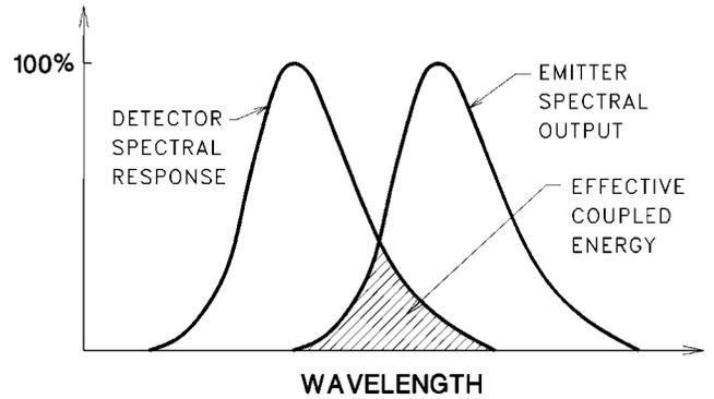
The LED/photocell matching factors listed are independent of power output from the LEDs. In order to get a real feel on how well any LED/photocell pair couple together, the power output from the LED at a particular forward drive current must be considered.
