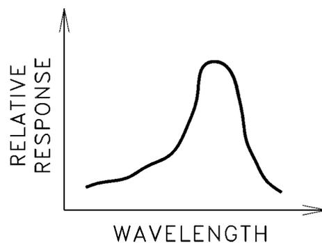
The spectral response curves for PerkinElmer's material types are given in the handbook and should be considered in selecting a photocell for a particular application.
