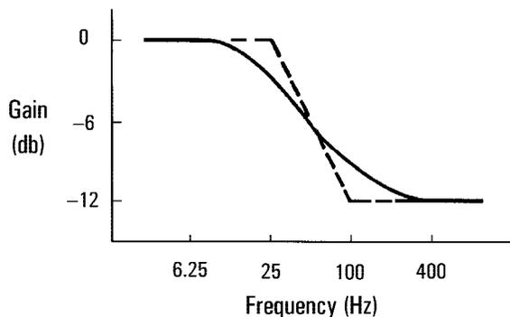
Figure 8b. Amplitude vs. Frequency for the Amplifier
