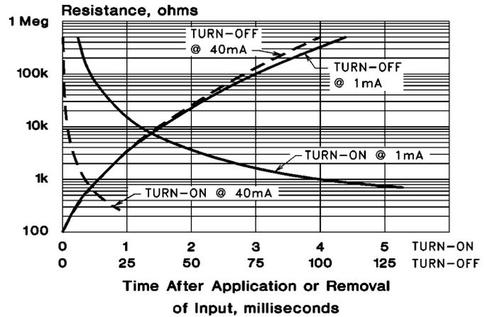
Output Resistance vs. Input Current
