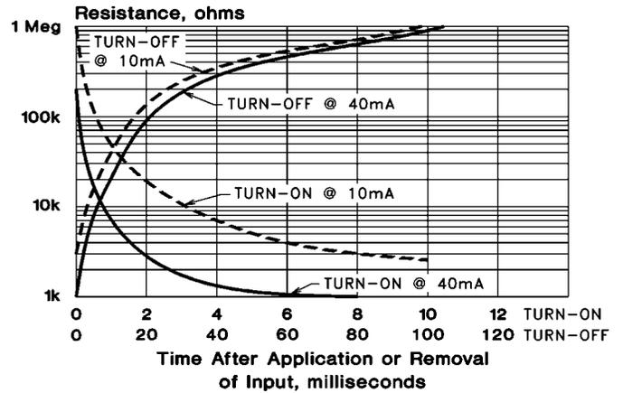
Output Resistance vs. Input Current
