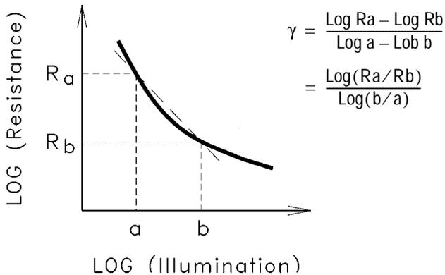
Applications for photocells are of one of two categories: digital or analog. For the digital or ON-OFF types of applications such as flame detectors, cells with steep slopes to their resistance versus light intensity curves are appropriate. For analog or measurement types of applications such as exposure controls for cameras, cells with shallow slopes might be better suited.
