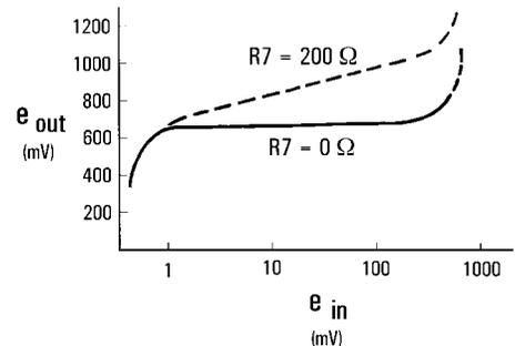
Figure 4b. Output Characteristics
