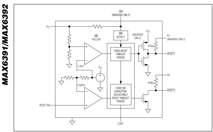
Figure 1. Functional Diagram
