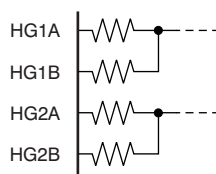
Figure 29. HG Double Power Connection
