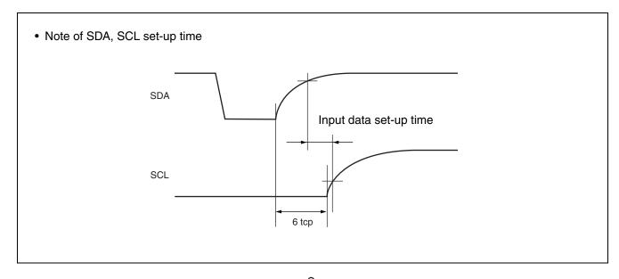
Note: The rating of the input data set-up time in the device connected to the bus cannot be satisfied depending on the load capacitance or pull-up resistor.
