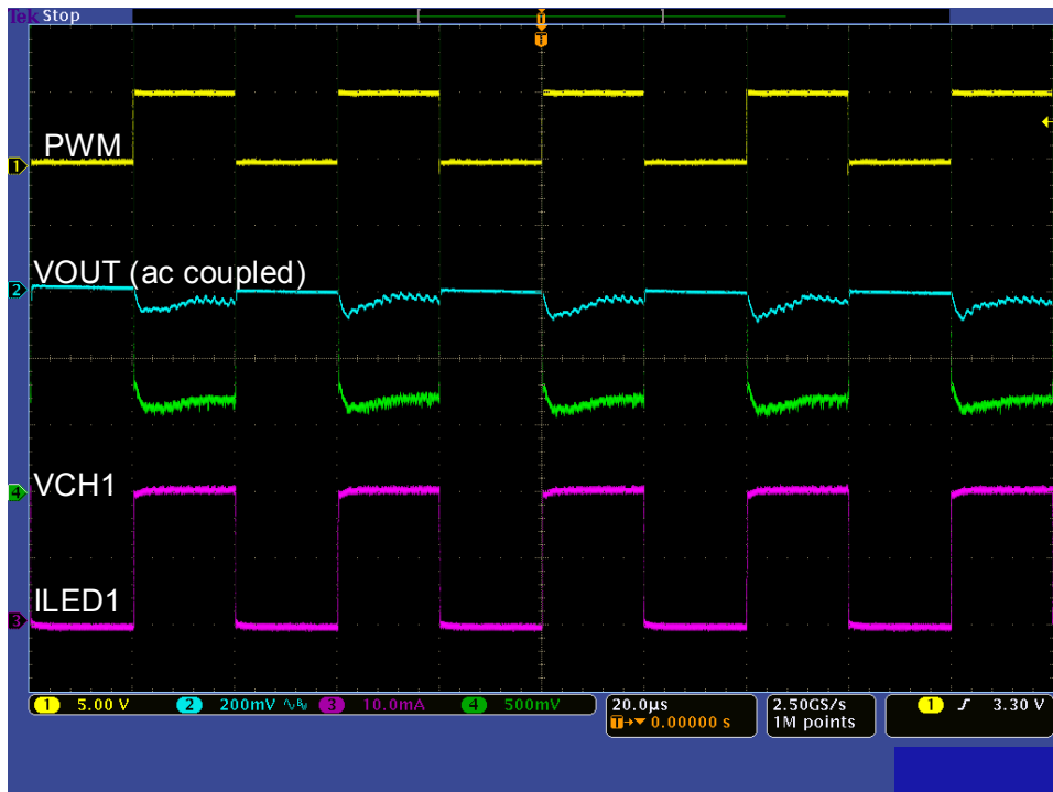
Figure 8. Typical Operating Waveforms (FPWM = 25 kHz, 50% duty)
