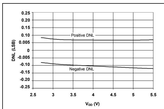
**FIGURE 2-12:** DNL vs.  $V_{DD}$  - I<sup>2</sup>C Fast Mode ( $f_{SCL} = 400$  kHz).
