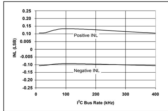
**FIGURE 2-4:** INL vs. Clock Rate ( $V_{DD} = 2.7V$ ).
