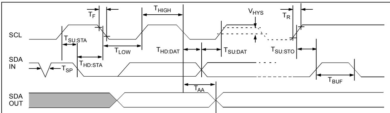
**FIGURE 1-1:** Standard and Fast Mode Bus Timing Data.
