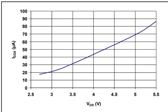
**FIGURE 2-33:**  $I_{DDA}$  (Active Bus) vs.  $V_{DD}$ .
