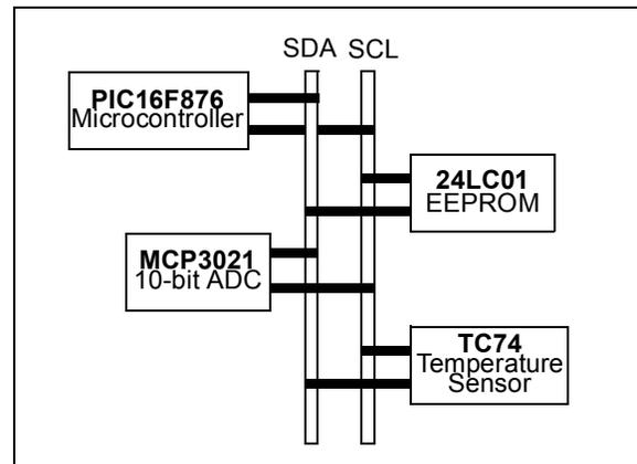
FIGURE 6-3: Multiple Devices on I<sup>2</sup>C Bus.
