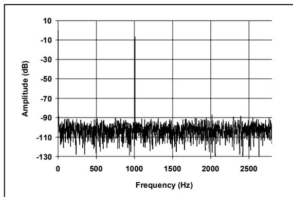
**FIGURE 2-29:** Spectrum Using I<sup>2</sup>C Standard Mode (Representative Part, 1 kHz Input Frequency).
