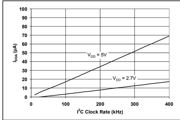
**FIGURE 2-34:**  $I_{DDA}$  (Active Bus) vs. Clock Rate.
