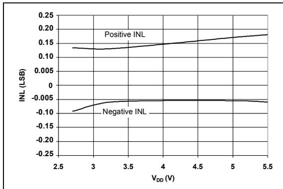
**FIGURE 2-2:** INL vs.  $V_{DD}$  - I<sup>2</sup>C Standard Mode ( $f_{SCL} = 100$  kHz).
