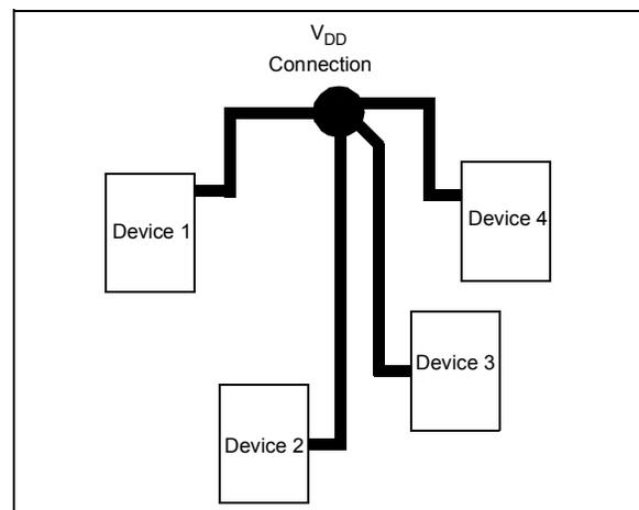
**FIGURE 6-6:** V<sub>DD</sub> traces arranged in a ‘Star’ configuration in order to reduce errors caused by current return paths.
