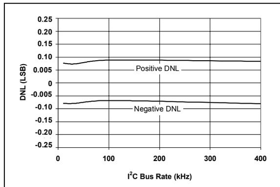
**FIGURE 2-11:** DNL vs. Clock Rate ( $V_{DD} = 2.7V$ ).
