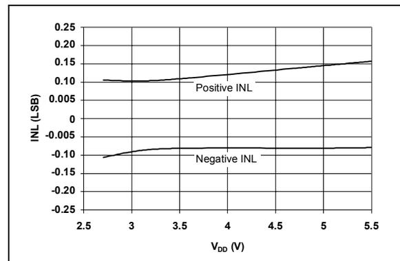
**FIGURE 2-5:** INL vs.  $V_{DD}$  - I<sup>2</sup>C Fast Mode ( $f_{SCL} = 400$  kHz).
