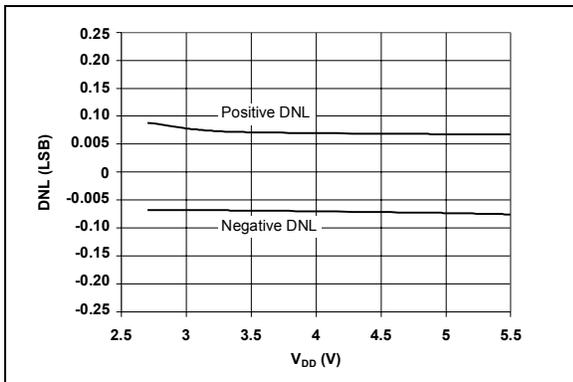
**FIGURE 2-9:** DNL vs.  $V_{DD}$  - I<sup>2</sup>C Standard Mode ( $f_{SCL} = 100$  kHz).
