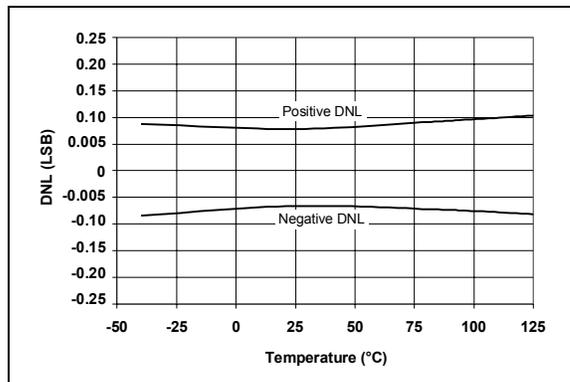
**FIGURE 2-17:** DNL vs. Temperature ( $V_{DD} = 2.7V$ ).
