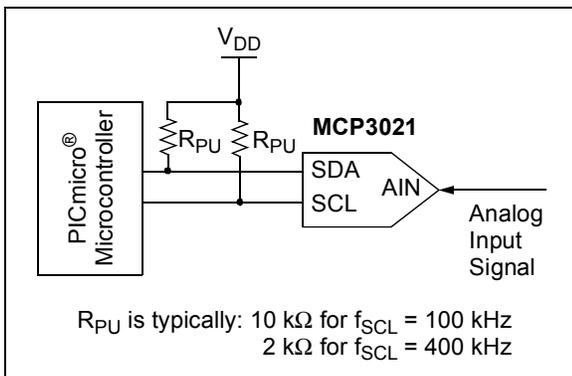
FIGURE 6-2: Pull-up Resistors on I<sup>2</sup>C Bus.
