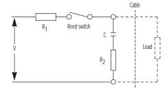
The above diagram illustrates a resistor/capacitor network for protecting a Reed Switch against high inrush currents.  $R_1$  and/or  $R_2$  are used depending upon circuit conditions.
