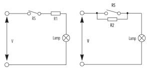
Lamp load with parallel or current limiting resistor across the switch
