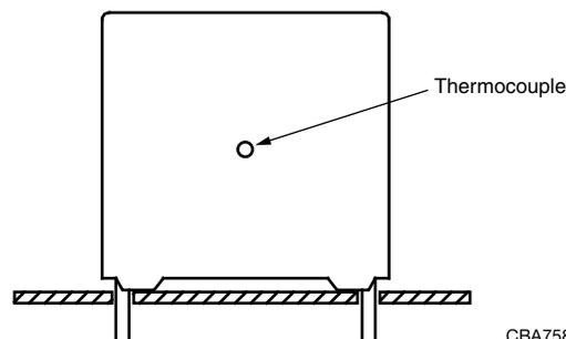
The temperature is measured in unloaded ( $T_{amb}$ ) and maximum loaded condition ( $T_C$ ).
