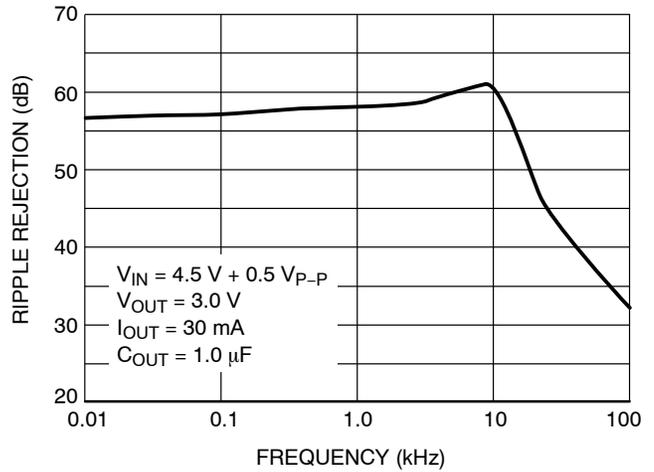
Figure 7. Ripple Rejection/Frequency
