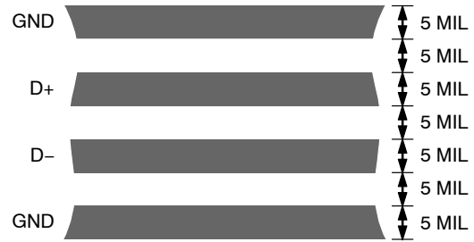
Figure 4. Typical Arrangement of Signal Tracks
