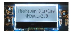
8. The NHDev display will then show "Press UP to select type". Pressing the UP and DOWN buttons will cycle through the available display categories that NHDev is programmed to demonstrate. Pressing the SEL button will enter that category and begin listing specific part number models.
