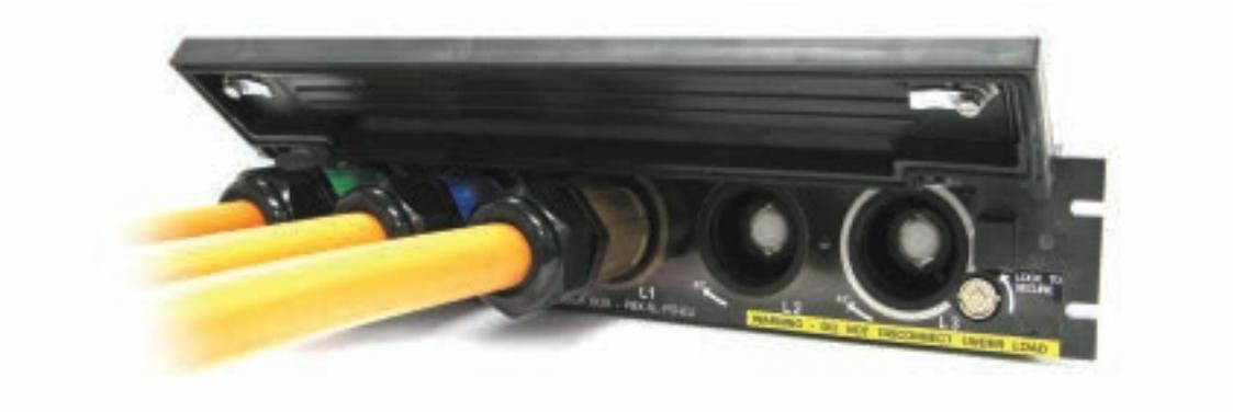
A PowerLock Box is a 3 phase high power connecting unit, used as a termination point for power cables. The boxes include a number of safety features to prevent incorrect connection and disconnection. All PowerLock devices are 'keyed' to eliminate the possibility of connecting with the wrong line, and color coded to suit international 3 phase standards.
