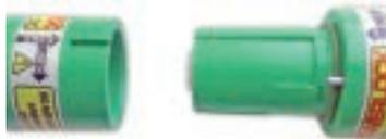
Uncoupled - Note the secondary locking pin on the right hand connector and the slot on the left hand connector.
