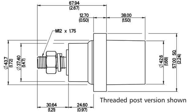
Panel Source connectors are supplied fully assembled with the male contact having an M12 threaded post, with nut and spring washer for connection to a standard cable lug, or M12 threaded hole for fixing with a bolt. These connectors are rated either 400 amp (T4 / H4) or 660 amp (T6 / H6).
