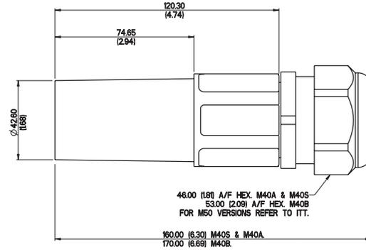
Line Source is the connector with a male contact which is normally connected to the source of the power. The contacts are fitted with a plastic end cap that prevents accidental finger touching of live parts of the connector and meets IP2X requirements. Different contacts are available to suit cable conductors from 25 mm<sup>2</sup> to 300 mm<sup>2</sup>.
