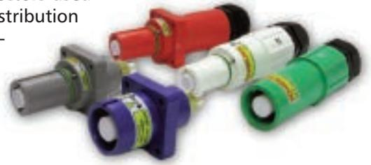
PowerLock connectors are easy to terminate to copper cable using either industry standard crimp tools or set-screw contacts. The silver plated contacts are available in 2 continuous current ranges, those with brass contacts are suitable for use up to 400 amps and those with copper contacts up to 660 amps.
