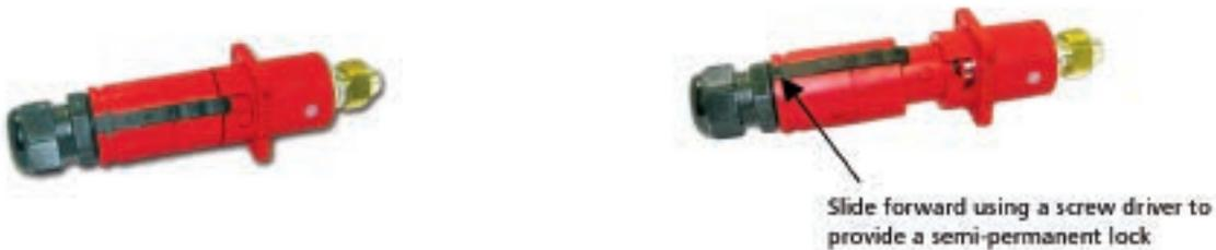
The spring loaded slide lock feature shown above locks into bayonet groove on the mating half, and can be disengaged by sliding back using ones thumb. This lock feature can be made semi-permanent by sliding the retainer forward.
