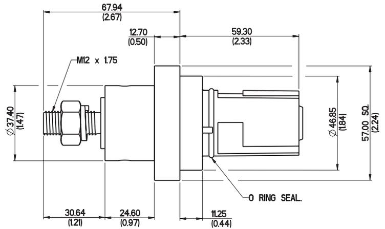
Panel Drain connectors are supplied fully assembled with the female contact having an M12 threaded post, with nut and spring washer for connection to a standard cable lug. These connectors rated either 400 amp (T4) or 660 amp (T6). This connector is fitted with the secondary locking pin for secure connections, see explanation on Line Drain page 13.
