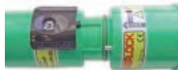
With the release key holding the locking pin back, the connectors can now be turned counter-clockwise and uncoupled.
