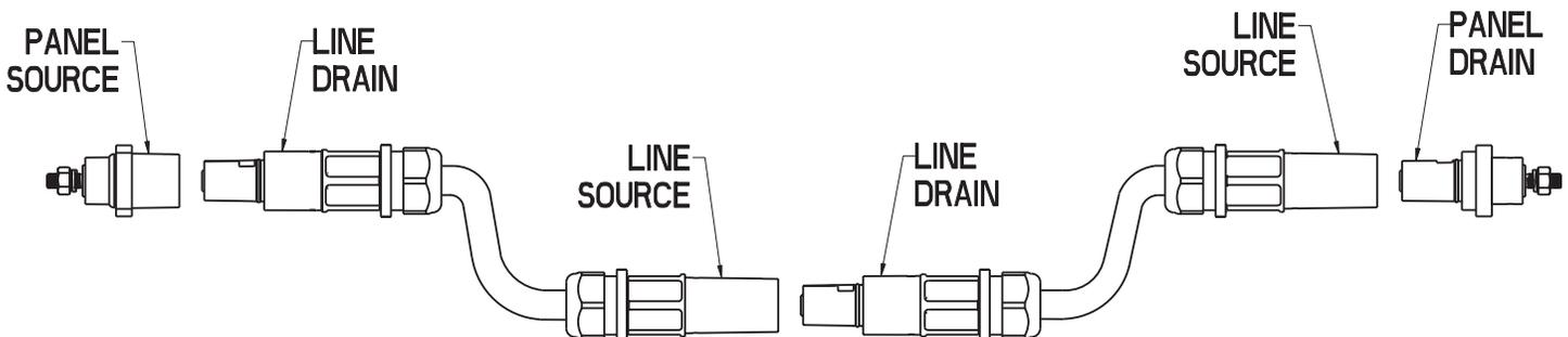
PowerLock connectors feature a bayonet coupling mechanism with a secondary locking pin. When a pair of connectors are mated and fully turned to engage the bayonet, the spring loaded secondary locking pin on the Drain connectors, snaps into a slot on the Source connector; a special release key is then required to uncouple the connectors.
