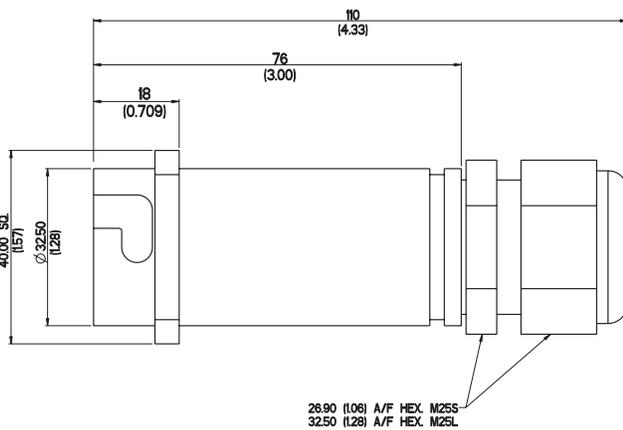
**Female Panel Socket with cable fixing**
