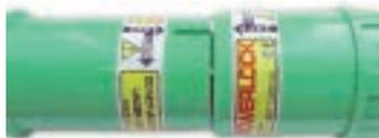
Aligning the arrow lines up the keyways allowing the connectors to be pushed together fully compressing the locking pin.
