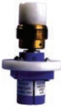
This device allows for direct connection of a generator cable to a 200A transformer pole mounted fuse unit. The existing fuse unit is unscrewed from the holder and replaced with the PowerLock unit, which incorporates a dummy fuse to allow for the outgoing circuit only. This enables the generator feed cable to be directly plugged into the pole mounted unit in order to feed the overhead Low Voltage transmission lines.
