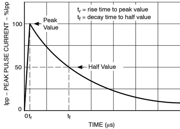
Figure 3. Nonrepetitive On-State Impulse vs. Waveform ( $I_{PPS}$ )
