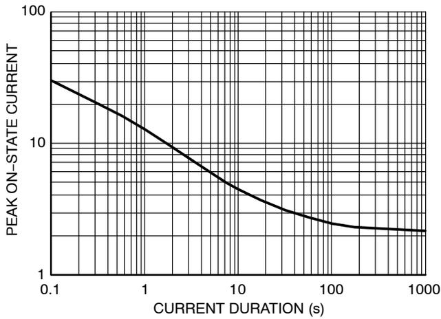
Figure 2. Nonrepetitive On-State Current vs. Time ( $I_{TSM}$ )
