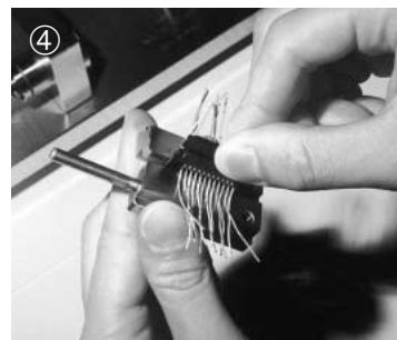
6. Pull down the handle. The wiring and cutting of excess cable length are completed.
