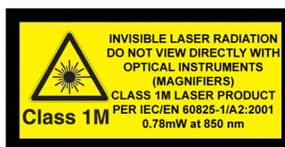
Additional laser safety information can be found on the Optek website. See application bulletin #221. Classification is not marked on the device due to space limitations. See package outline for center-line of optical radiance. Operating devices beyond maximum rating may result in hazardous radiation exposure.
