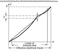
The independent linearity (conformity for the non linear laws) is the maximum gap  $\Delta V$  between the actual variation curve and the theorical variation curve the nearest to it. The linearity and the conformity are expressed in percentage of the total applied voltage E
