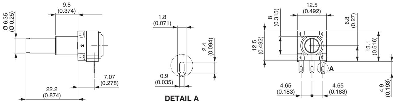
Single module, single shaft, vertical mounting, PC pins with support plate, imperial bushing and shaft
