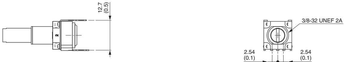
Single module, single shaft, solder lugs, imperial bushing and shaft
