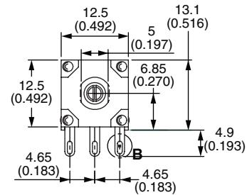
Single module, single shaft, vertical mounting, PC pins with support plate, metric bushing and shaft
