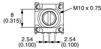
Dual modules, single shaft, PC pins with front support plates, imperial bushing and shaft
