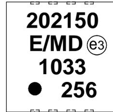
8-Lead DFN-S (6x5x0.9 mm)
